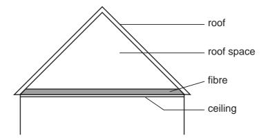
Heat cannot easily escape through the ceiling because the fibre
