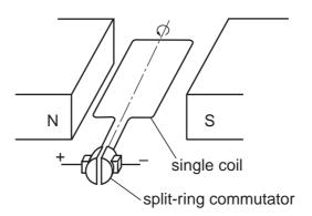
The split-ring commutator reverses the current in the coil as it rotates.
