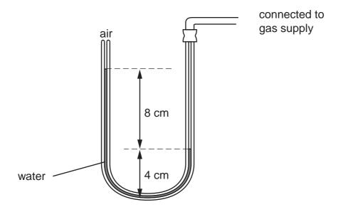
Pressure can be measured in cm of water.
